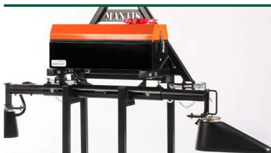
Time-dependent metering via an electric pump
