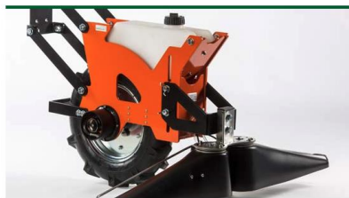
Path-dependent metering via a wheel-driven pump
